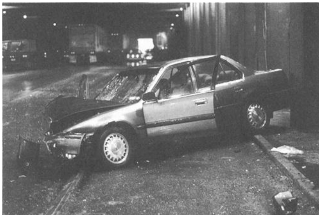
FIG. 3—An imported compact car with severe front end damage following impact with wall.
